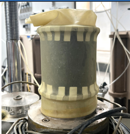
Lubricated Ends Triaxial Tailing Specimen
